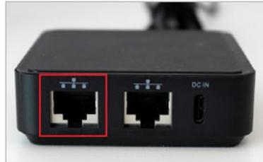
10. Plug the SkyTab POS power cable into the DC IN port on the USB Hub. Plug the other end of the power cable into a wall outlet.
